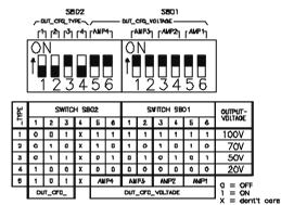
diagram 7 Output configuration settings of the amplifiers (rear view)
